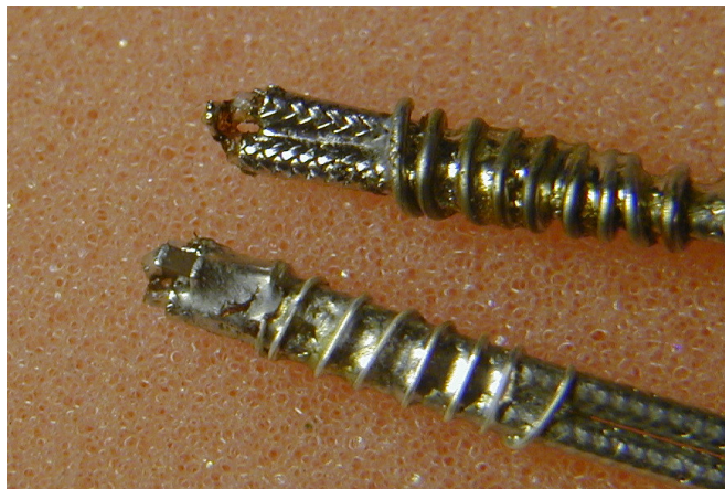
Figure 8: Low inductance measurement fixtures without (top) and with (bottom) a capacitor mounted as the DUT.
